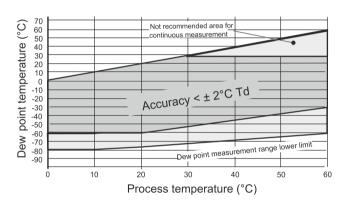
DEW POINT ACCURACY VS. MEASUREMENT CONDITIONS
