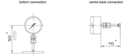
\*The necktube is extended by 36 mm for thermometers without capillaries and with scale ranges ≥160°C
